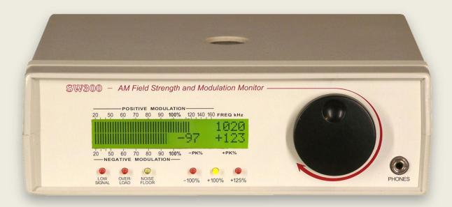
The Schlockwood 300 (SW300) is a compact, portable field strength meter and modulation monitor for medium-wave AM broadcast applications. It satisfies needs ranging from those of Part 15 operators to commercial stations.
