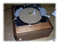
covered with a rubberized cork material. Also visible is the 2-piece spindle adapter for the 15mm CD/DVD center hole, machined as a favor by a friend. The loose piece screwsdown over the other to clamp the disc so it won't slip on the turntable.
