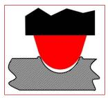
ed recording, the horns more or less flowed into place and the high frequency detail is not as well defined in embossing as in the engraved groove. The horns are also somewhat fragile, so the recording won't deliver as many plays before the sound quality degrades.
