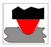
So, what about a stylus exactly the same size and shape as the recording stylus? Yes, that might help, but embossing a groove by applying high pressure at the stylus tip is a 'fluid' process, and the material tends to spring-back and even shrink after it is deformed in passing under the recording stylus. Therefore actual groove geometry is neither very predictable nor well defined. A slightly oversized playback stylus does yield better sound.
